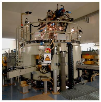
A high-energy multi-particle cyclotron for scientific research and production of innovative radionuclides for medical use
